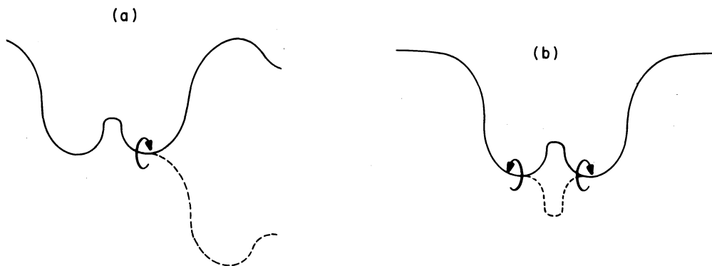
Fig. 1. Schematic representation of conformational transitions in polymer chains. (a) A single rotation around a bond in the chain backbone. (b) Two correlated rotations in a crankshaft-like motion.
